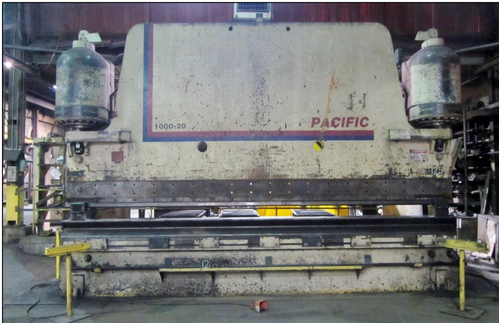
PACIFIC 1000-20 20' X 1000 TON HYDRAULIC PRESS BRAKE
