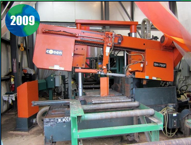
COSEN SH-760F HORIZONTAL STRUCTURAL STEEL BANDSAW
