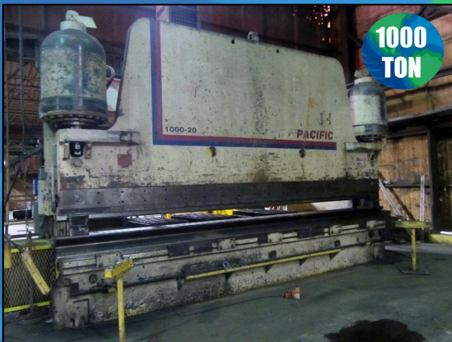
PACIFIC 1000-20 20' X 1000 TON HYDRAULIC PRESS BRAKE
