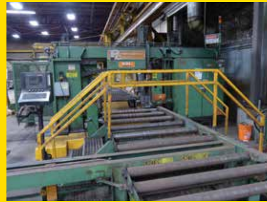
PEDDINGHAUS BDL1250/9A Beam Drill w/27" x 40" Infeed / Outfeed Conveyor
