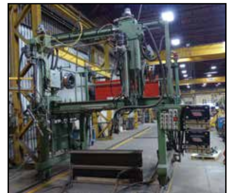
OGDEN DART IV Automated Sub Arc Seam Welder
