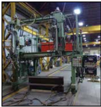
OGDEN DART IV Automated Sub Arc Seam Welder
