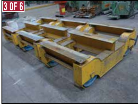
(6) Rail Transfer Carts
