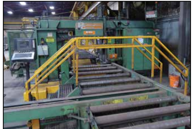
PEDDINGHAUS BDL1250/9A Beam Drill w/27" x 40" Infeed / Outfeed Conveyor
