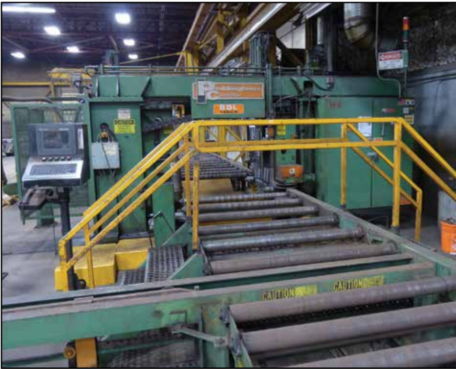
PEDDINGHAUS BDL1250/9A Beam Drill w/27" x 40" Infeed / Outfeed Conveyor
